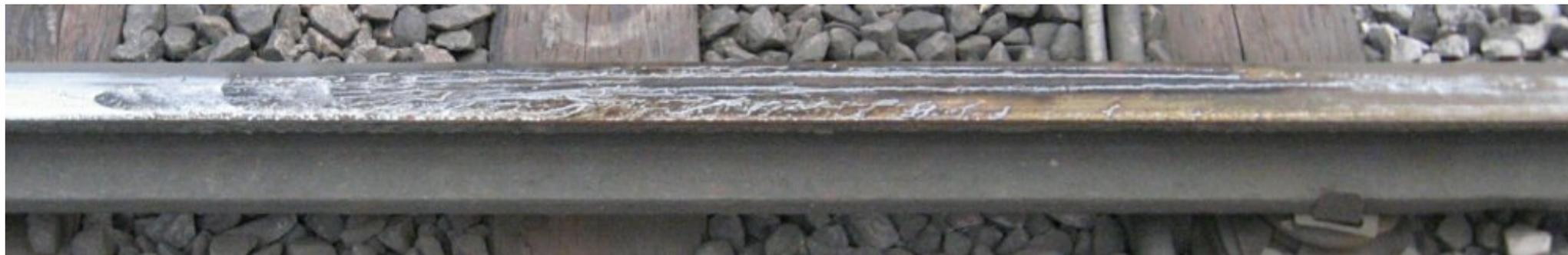
*A VRG - arcing on the negative rail - most negative shoes will not pick up current when travelling over this.*
