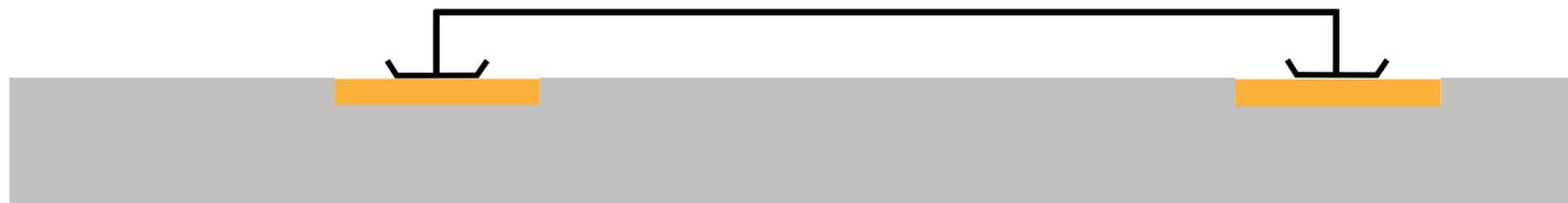
*Two Virtual Rail Gaps on the negative rail - both shoes are off traction current*
