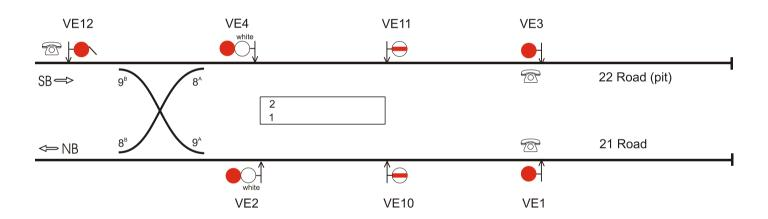
The diagrams on the following pages show the tracks between Kings Cross and Warren Street with the NB at the bottom and the SB at the top
